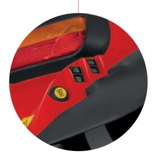
**Easy to reach:**External controls on both fenders for easy implement connection.
