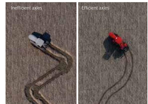
In comparison to a 2-track-system, the 4-track-system steers under full loads minimizing soil disturbance when turning.
