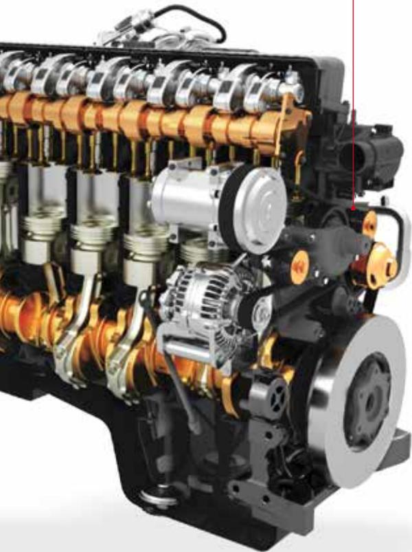
Delivering the highest power output in their class, Case IH Steiger and Quadtrac tractors are powered by a high pressure common rail 12.9 litre FPT engine featuring a two-stage turbo and newly-developed cooling system.
